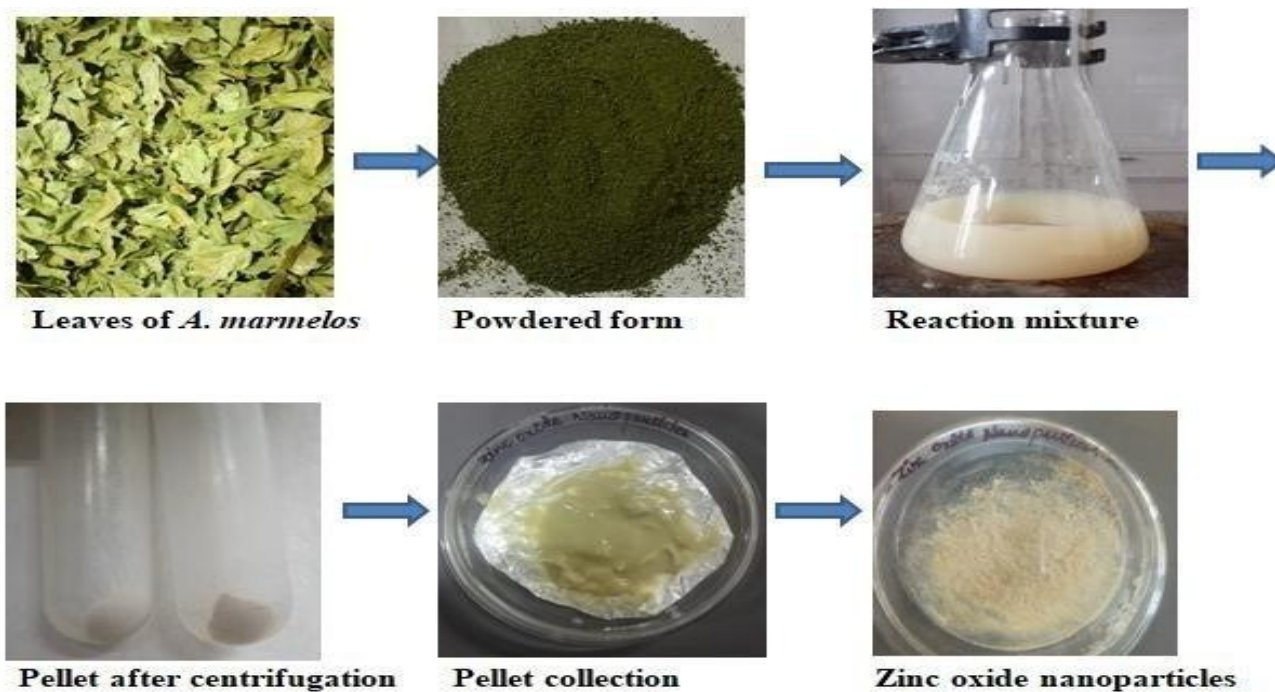
Fig. 4. Green synthesis of ZnONPs using A. marmelos leaf extract
