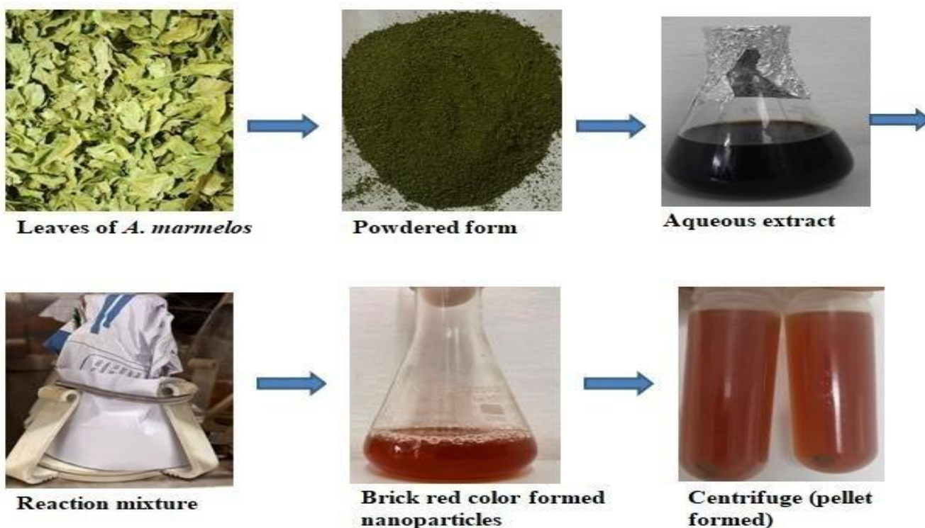
Fig. 5. Green synthesis of \text{SeO}_2\text{NPs} using A. marmelos leaf extract
